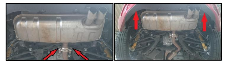
3. The middle pipe need to be shortened – cut off 25cm measured from the flanche (see the photo)
