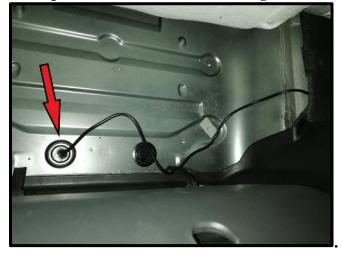
7. Get the wire out for approx. 60cm. Hide the wire behind the heat shield.
