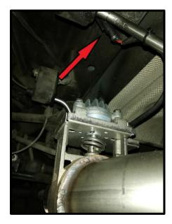
12. Check that the valve reacts on pressing the remote control buttons.
