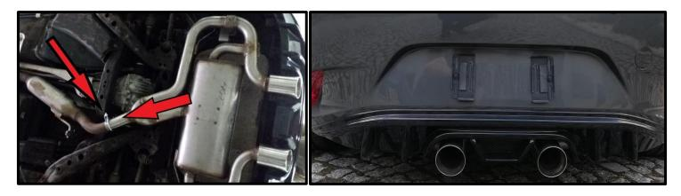
11. Connect the central unit wire with the exhaust valve.
