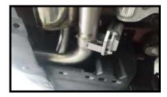
10. Test the RC operation – pressing the button should trigger the electric valve.
