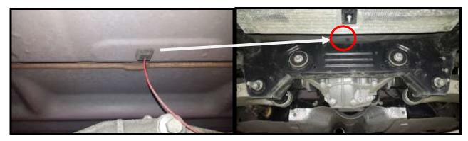
6. Connect the other end of the cable to the 12V socket (inside the vehicle)
